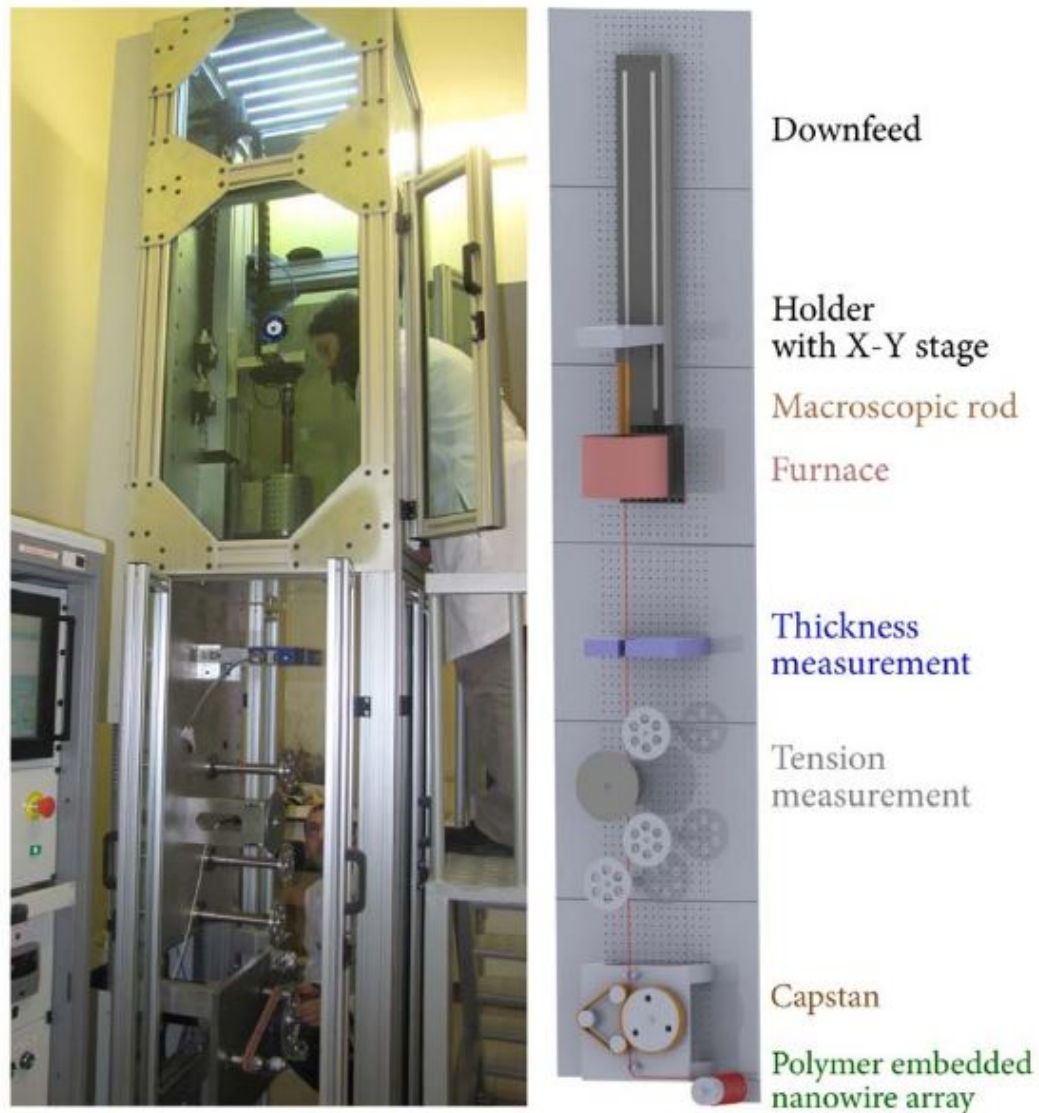
Figure 4.2: Fiber tower for the drawing process and the corresponding components of the fiber tower [67]
