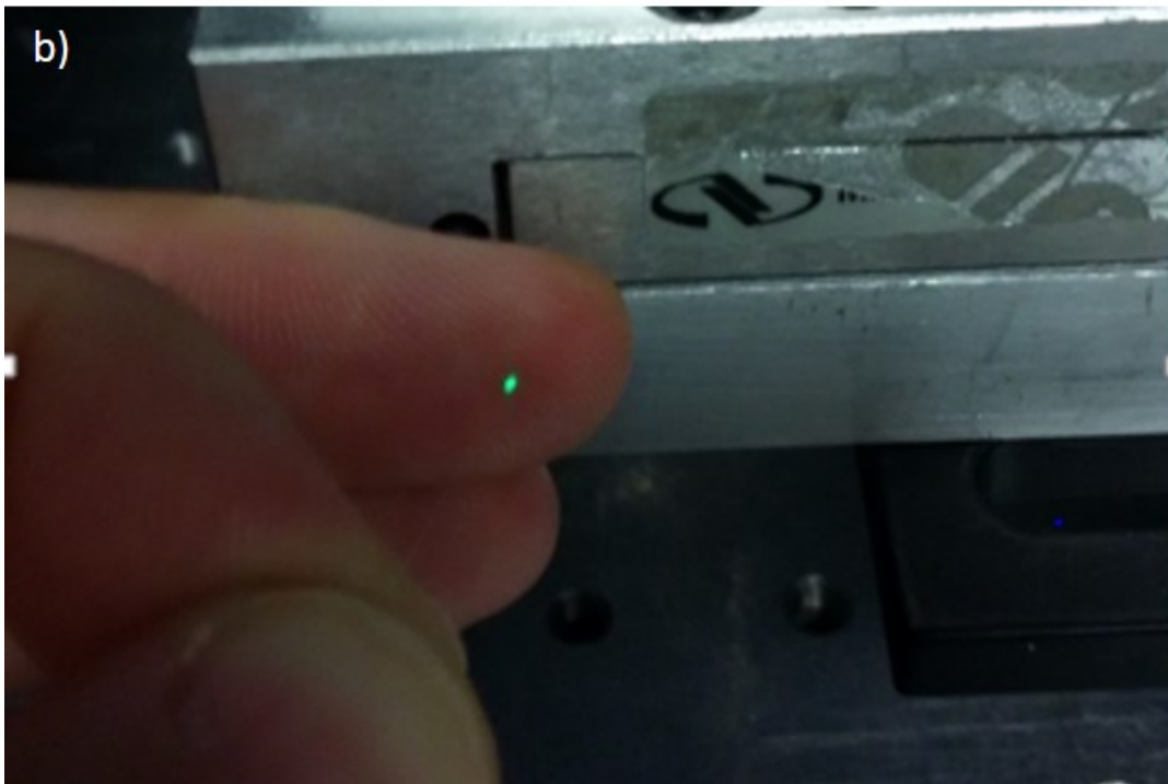
Figure 3.11: a) Visible green light observed during SCG process in the fiber before tapered chalcogenide fiber got splitted, b) and at the fiber tip after it got splitted.
